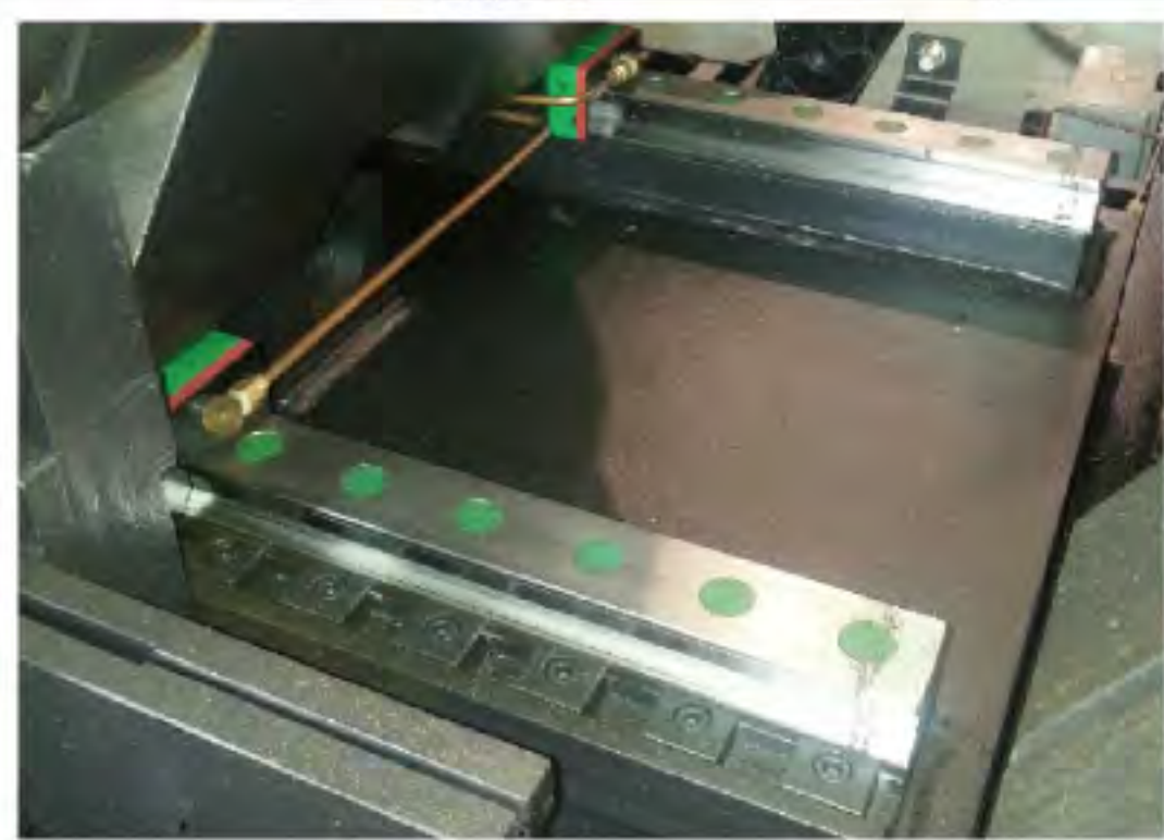
The saw head is ball screw actuated with premium grade linear guide ways.(P-230B)
