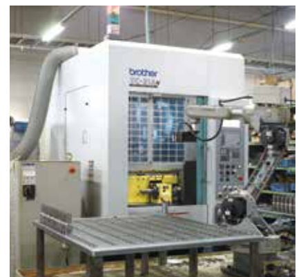
CNC table on TC-31A(pallet changer)+ component-change by robot
