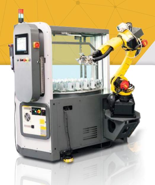
With the Cubebox Blues RT, you can create more stock space by stacking diameter parts on top of each other and can integrate long shaft parts into the automation system.
