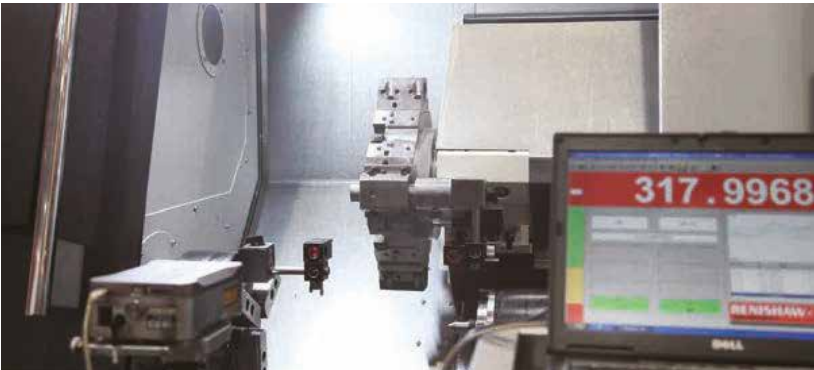
• Laser interferometer testing to guarantee the all axes' precision.
