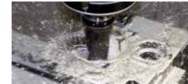
Machining details Holediameter: D40 mm Material: Carbon steel
