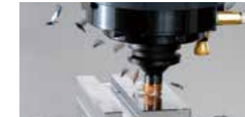
Machining details Cutting amount: 110 cc/min Material: Carbon steel (using D16 end mill)
