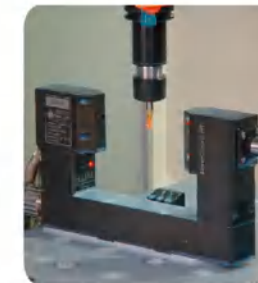
■ Tool Length measurement system
